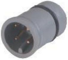
M12 Insert Sensor/Actuator Receptacle Connector: Male, insert with O-ring, M12 - mating side, solder contacts - connecting side, 4-pin, A-coded, unshielded, grey body, 150 V AC/DC, 4 A
